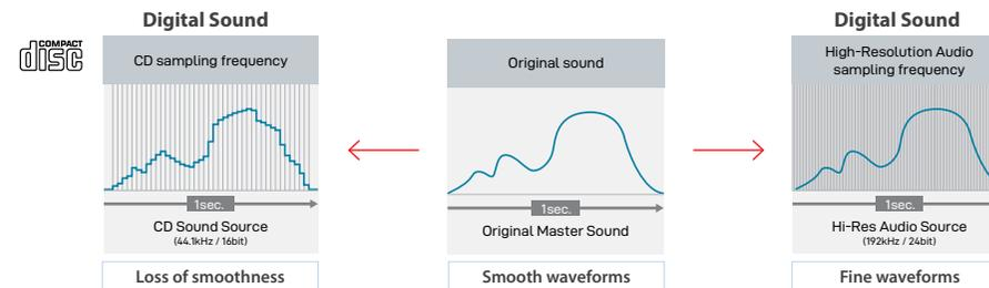
Both CD and Hi-Res Audio are digitized versions of the actual sound; Hi-Res Audio is able to digitize and store the sound in more detail than CD, so the waveform of the sound is closer to the original sound. Hi-Res Audio has 6.5 times more information than standard CD quality.
