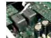
for subwoofer prevents magnetic flux from radiating from the coil and reduces noise resulting in high quality sound.
