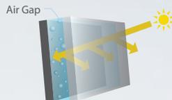
Glare is decreased by removing the air gap using Optical Clear Adhesive (OCA).
